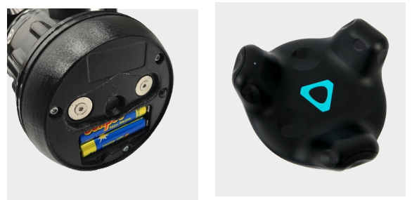
Figure 16: When installed, the puck should look like this
