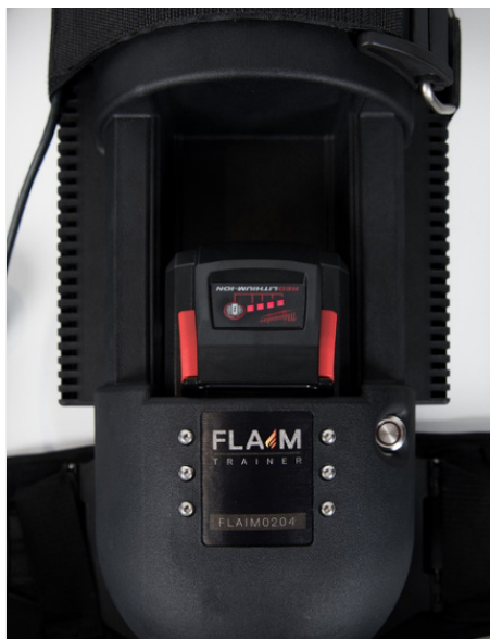
Figure 20: Step 4. Power on SCBA Backpack - short press- short press
