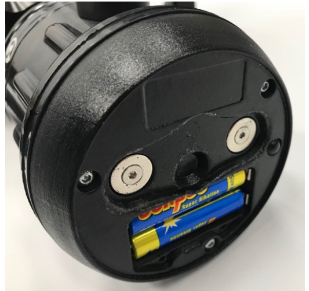
Figure 50: Nozzle batteries behind tracking puck
